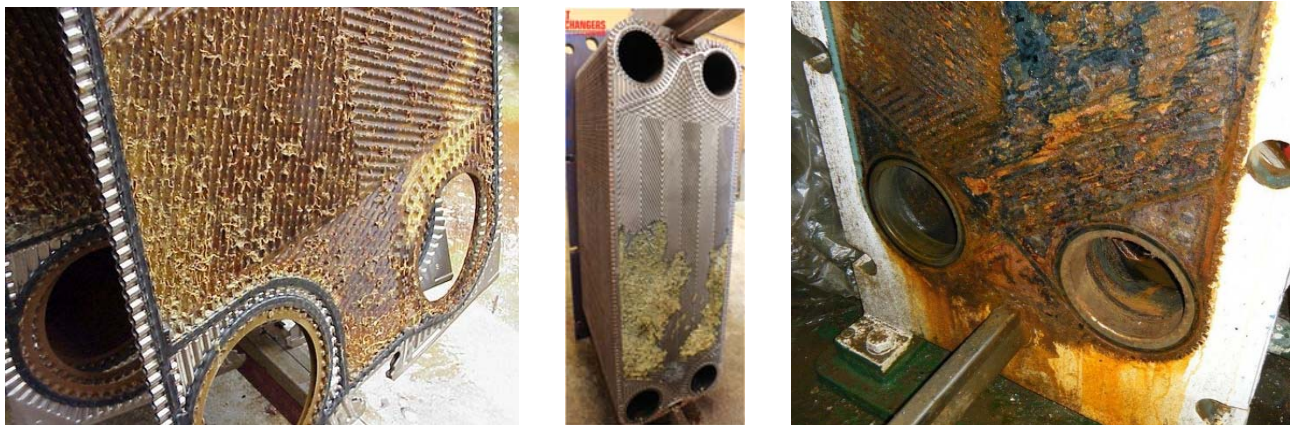
Figure 1 Scaling on Frame and Plate Heat Exchangers
